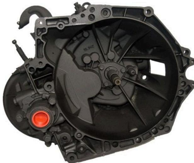
Ivor Searle has expanded its comprehensive remanufactured programme by adding the five-speed manual gearbox for the Citroën Dispatch and Peugeot Expert light vans. This new unit covers the third-generation, 1.6-litre, 95 bhp diesel models manufactured between 2016 and 2019.
