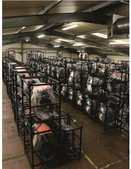
Part of the stock of remanufactured engines, wrapped and protected in their individual stillages
